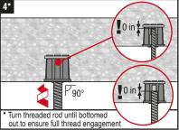
UL/FM Listing does not cover the 1/4 inch rod size
