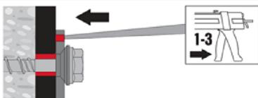
Fill the annular gap between screw and fixture with 1-3 strokes of a Hilti injection mortar HIT-HY ... or HIT-RE ....
