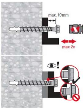
A screw can be adjusted maximum two times. The total allowed thickness of shims added during the adjustment process is 10 mm. The final embedment depth after adjustment process must be larger or equal than  $h_{nom2}$  or  $h_{nom3}$ .
