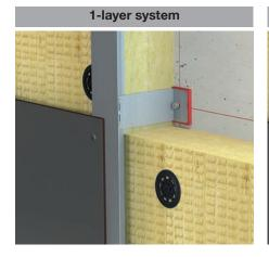
• Vertical bracket in line with the vertical profile.
