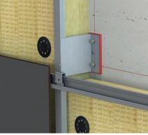
• Vertical bracket in line with the vertical profile for the 1<sup>st</sup> layer and the 2<sup>nd</sup> layer in horizontal alignment (2<sup>nd</sup> layer profiles with slotted holes for expansion compensation.)
