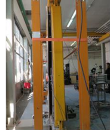
3. Out-of-plane collapse of panels without falling down of panels
