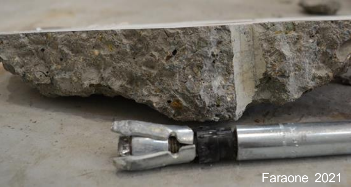
Expansion anchor following test
