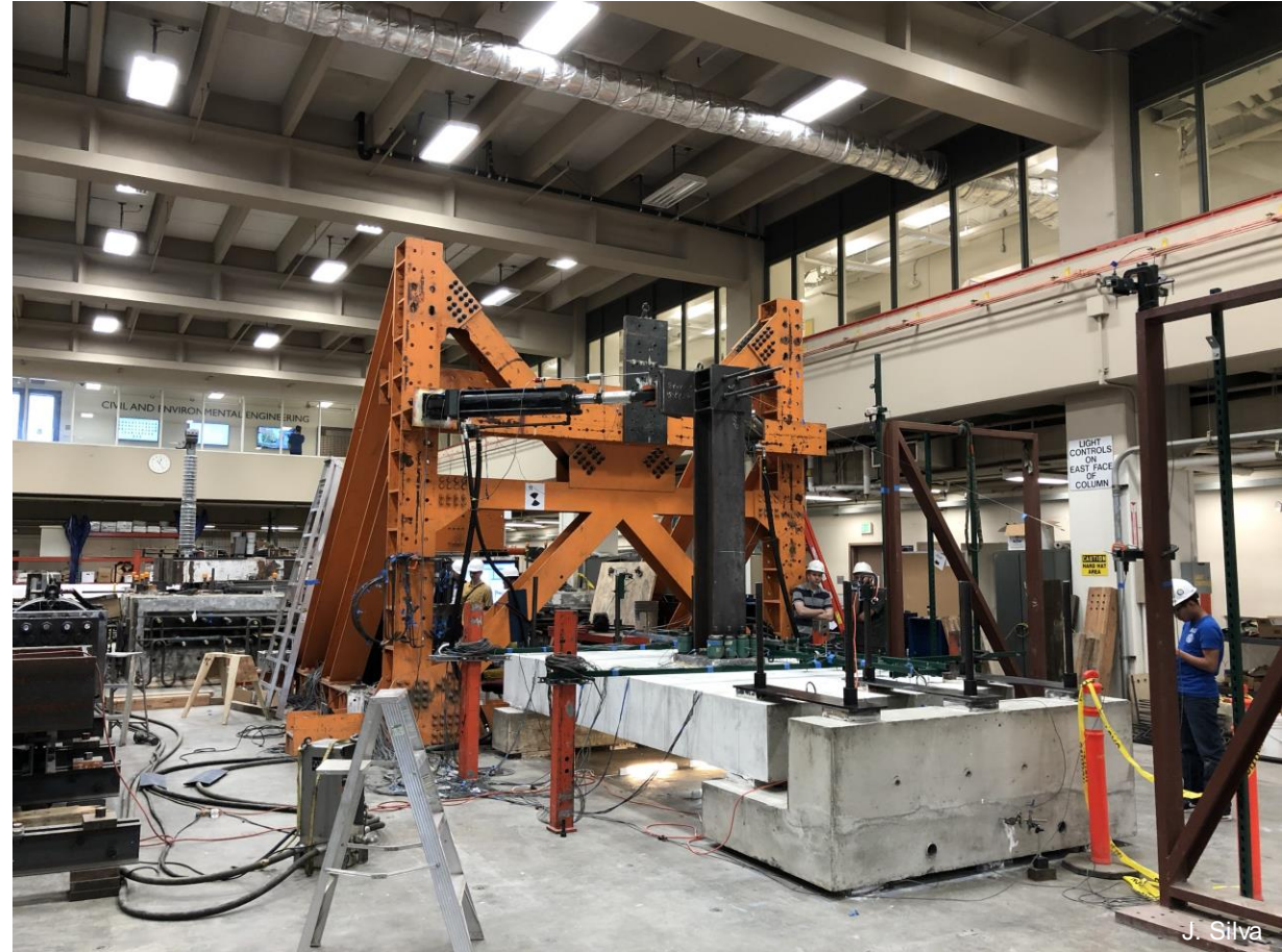
Column to foundation under applied moment and shear – full scale
