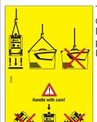
The power supply may be lifted by crane only at the lifting points provided. Never loiter in the vicinity of loads sus-
